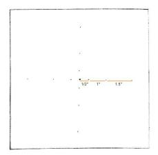
Next, measure out another distance from the center dot. Using the same process as before, make a mark at this same distance on top, below, to the left and to the right of the center dot.
