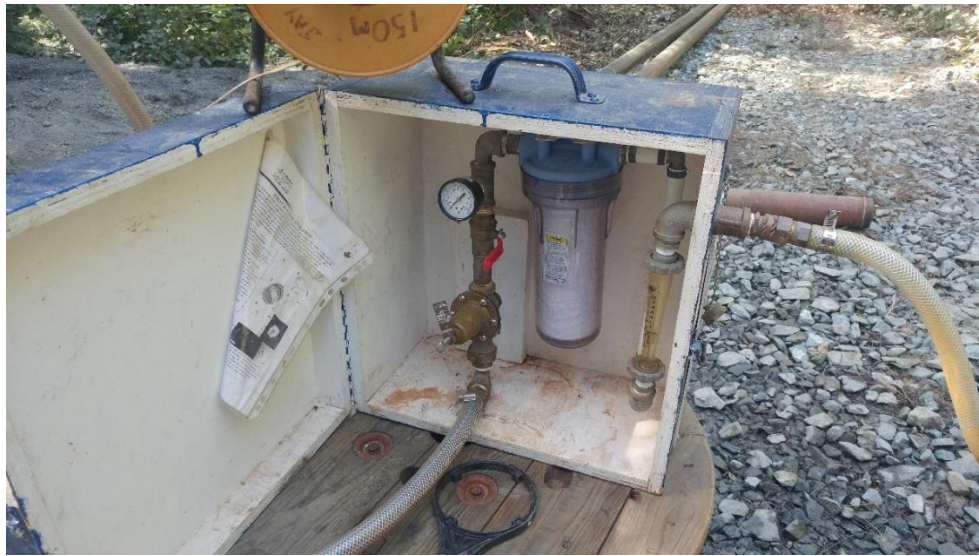
Photo A7: MPA filter during constant rate test; flow rate 355 m 3 /d (65.1 USgpm)
