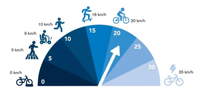
**Figure 1.1 Typical Speeds for Different Users** Source: Content by BC Active Transportation Design Guide
